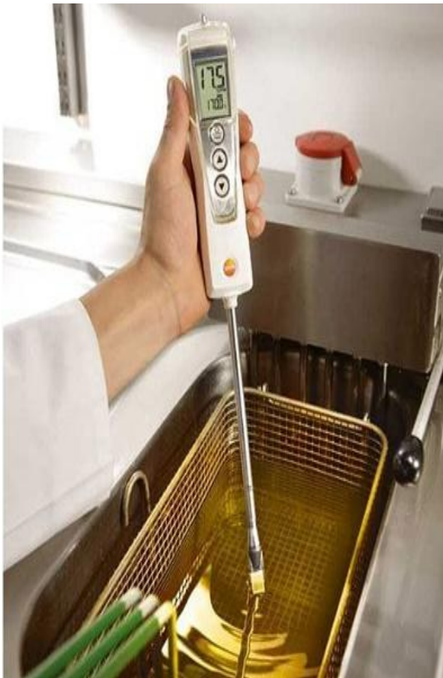
Figure 3: A Simple Device That Measures the TPM by EC
