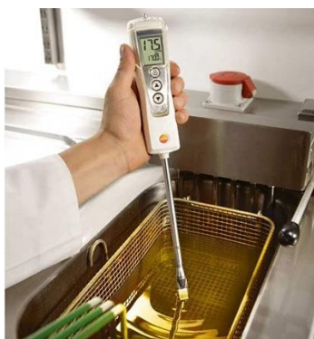
Figure 3- Simple device measuring the TPM by EC
